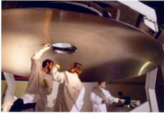
Machined mirror blank undergoing ultrasonic inspection of the brazed joints between its segments.
